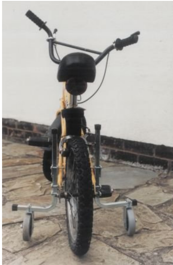
Standard adjustabilisers with stabiliser wheels at outer lateral positions
