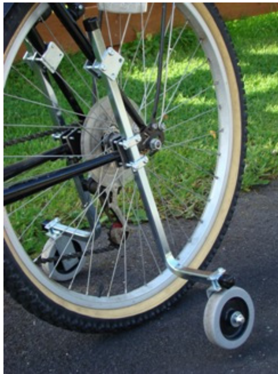
Large adjustabilisers with stabiliser wheels at outer lateral positions
